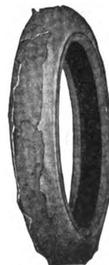
This is a worn out casing as it comes to us to be MADE NEW
